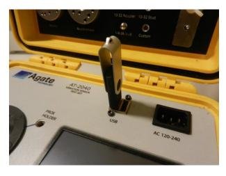
Figure 47. USB memory drive loaded in USB port
