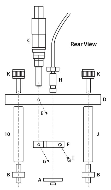
Figure 42. Rear view of the proximity probe kit installation
