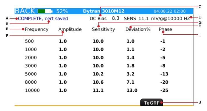
Figure 20. Automatic testing screen - table view
