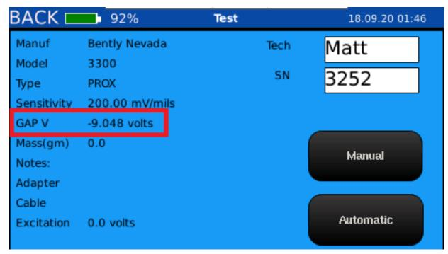
Figure 45. Sensor profile screen for the proximity probe
