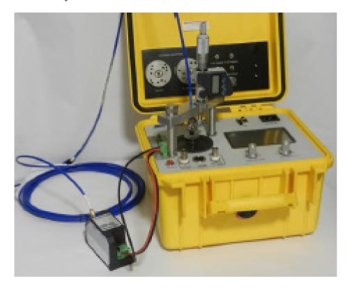
Figure 44. Proximity probe driver connected to AT2040
