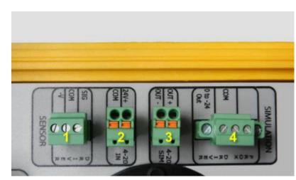
Figure 34. Connect the sensor to connector "2"
