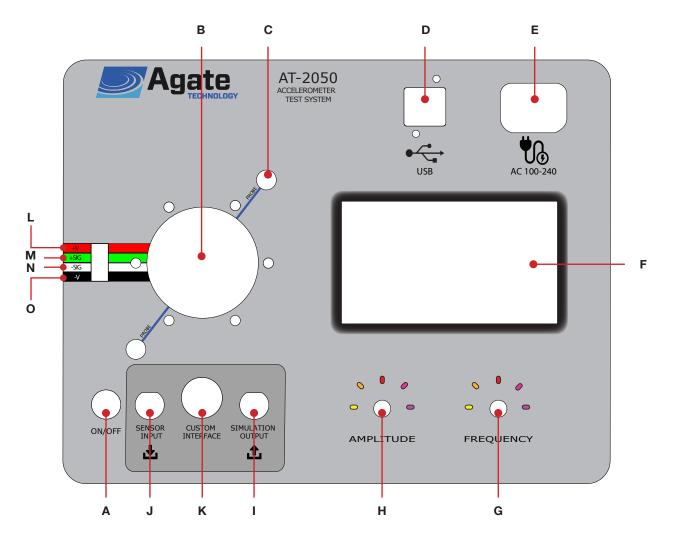
Figure 6. Physical diagram of the AT2050
