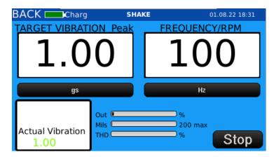
Figure 59. Default units showing on Shaker Screen
