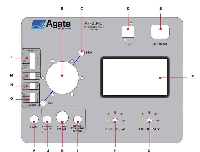
Figure 4. Physical diagram of the AT2040
