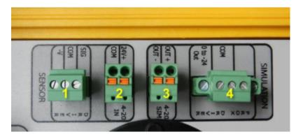
Figure 68. 4-20mA ("3") and proximity probe simulator connectors ("4")
