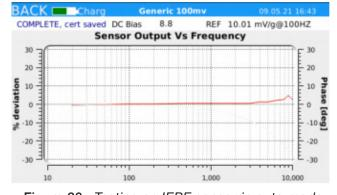
Figure 26. Testing an IEPE sensor in auto mode
