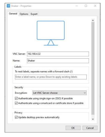
Figure 74. Enter IP address and name
