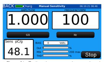
Figure 31. Testing charge sensor in manual mode
