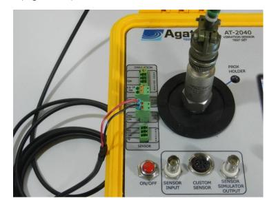
Figure 33. Sensor mounted to the AT2040
