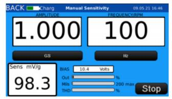
Figure 25. Testing an IEPE sensor in manual mode
