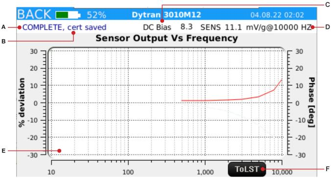
Figure 19. Automatic testing screen – graph view
