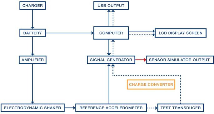
Figure 2. Block diagram
