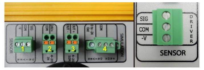
Figure 43. Proximity probe driver input
