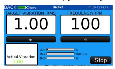
Figure 60. RMS units showing on Shaker Screen
