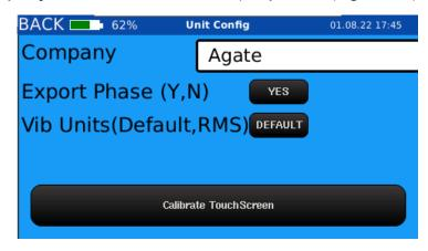
Figure 56. Enter company name, show/hide phase data, change output units, and calibrate touchscreen
