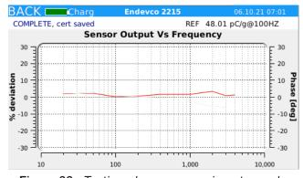
Figure 32. Testing charge sensor in auto mode
