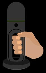
3. Take the device and start walking only when the initialization has finished and the LED turns green.
