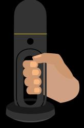
2. While initializing (LED blinking yellow) hold the device stable on the table stand.
