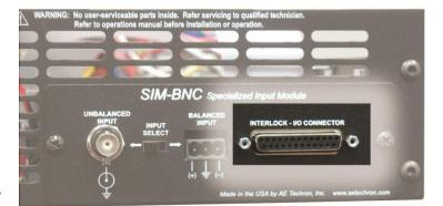
Figure 8.3 - Interlock I/O Connector
