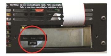
Figure 4.14 - Bi-Level Power Switch Location
