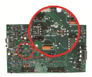
Figure 4.9- Stop Mode on OverLoad Setting
