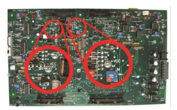
Figure 8.1- +Vcc and -Vcc Test Point Locations
