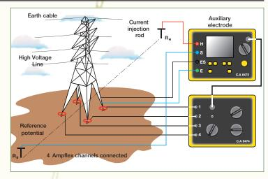
Used in conjunction with the Model 6474 vectorial processing unit, the Model 6472 offers the possibility of measuring a pylon's earth resistance even if it is part of a parallel earth network, by selective measurement of the pylon in question.
