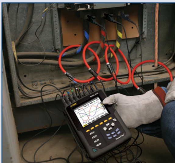
Power quality analysis on a three-phase panel using the AmpFlex® flexible current probes.
