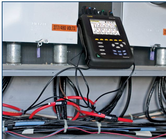
AmpFlex® flexible current sensors facilitate easy access to current carrying conductors.
