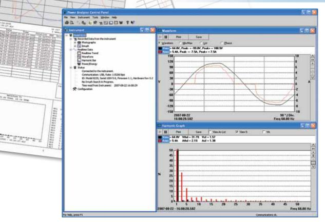
DataView® software provides a convenient way to configure and display power quality measurements from your computer. Through the use of clear and easy-to-use tabbed dialog boxes, all PowerPad® functions can be configured and tests can be initiated. Results can be displayed in real-time and stored in your PC. Reports may be printed along with the operator's comments and analysis.
