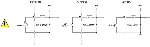
Fig. 14 - Voltage connection
