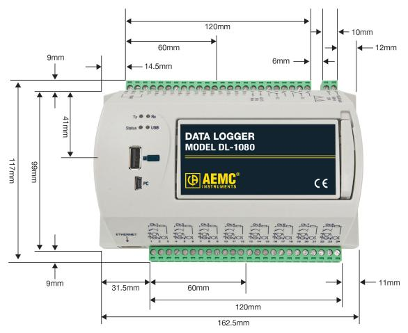
Fig. 04 – Dimensions without DISPLAY module
