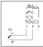
The Thermocouple connection for the channels is made to the terminals in accordance with the figure at the left. Please observe the correct connection polarity.
