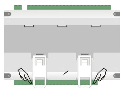
Fig. 01 - DIN rail installation
