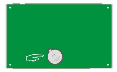
• Insert the new battery and reinstall the back cover and its four screws.
