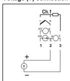
The voltage connection for the channels is made to the terminals in accordance with the figure at the left. Please observe the correct polarity of the connection.
