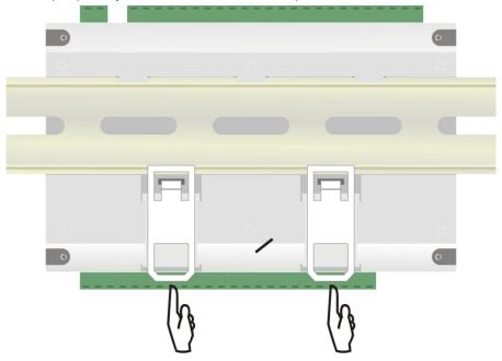
Fig. 03 - DIN rail installation
