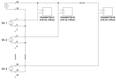
Fig. 19 – Auxiliary power supply powering 4-20mA (2-wire) transmitters
