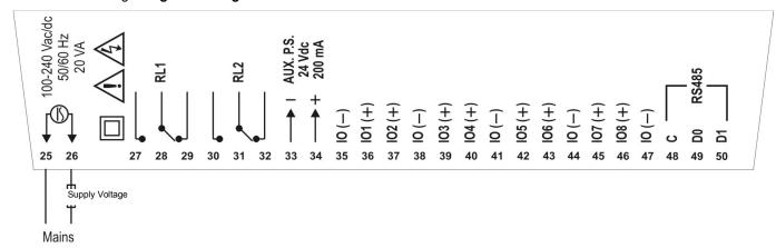
Fig. 12 - Upper side connections
