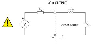
Fig. 17 - Connection of a load R<sub>L</sub> to a digital output
