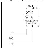
The millivolt connection for the channels is made to the terminals in accordance with the figure at the left. Please observe the correct polarity of the connection.
