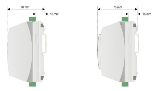
Fig. 05 – Dimensions of the side without DISPLAY module Fig. 06 – Dimensions of the side with DISPLAY module
