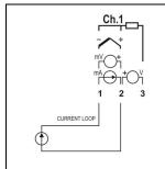
The milliamp connection for the channels is made to the terminals in accordance with the figure at the left. Please observe the correct polarity of the connection.
