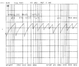
Figure 7-3. Fractional-N Tuning Voltage Waveform at Abus Node 21
