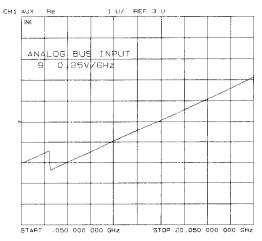
Figure 10-6. Node 9: 0.25V/GHz, Source Tuning Voltage
