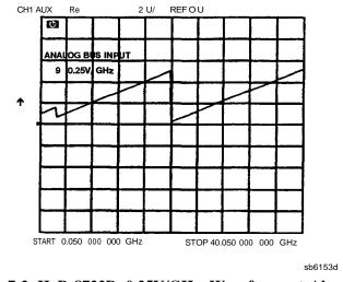
Figure 7-2. H P 8722D 0.25V/GHz Waveform at Abus Node 9
