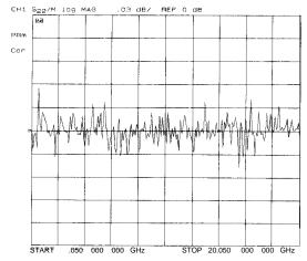
Figure 4-10. Typical Switch Repeatability Trace
