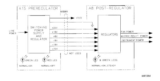
Figure 5-1. Power Supply Goup Simplified Block Diagram
