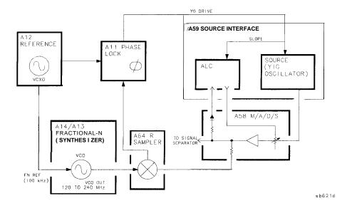
Figure 12-3. Source Functional Group, Simplified Block Diagram
