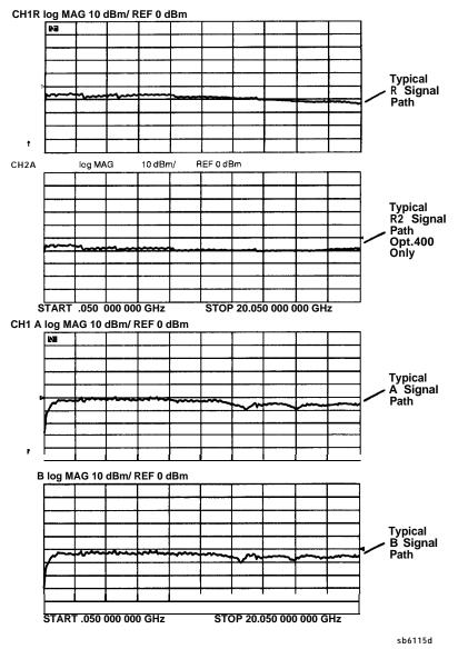
Figure 8-1. Typical R1, R2, A, and B Traces
