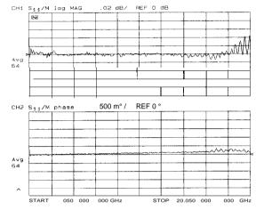
Figure 2-5. Cable Magnitude and Phase Stability
