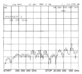
Figure 2-3. Return Loss Measurement of Cables
