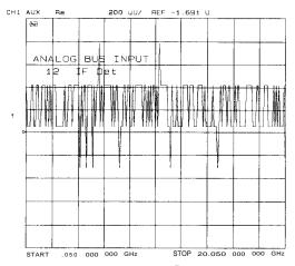
Figure 10-8 Node 12: Typical IF Detector Voltage Trace
