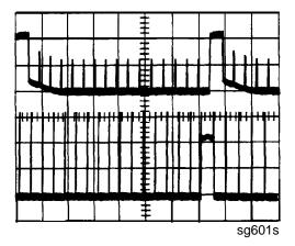
Figure 6-11. A7 CPU Walking One Pattern
