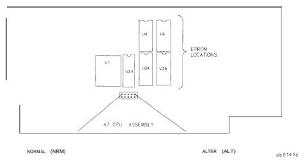
Figure 10-2. Jumper Positions on the A7 CPU
