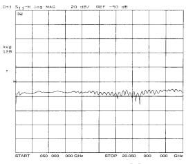
Figure 2-6. Connector Repeatability Example
