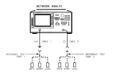
Figure 2-9. Connections for Measurement Calibration Standards
