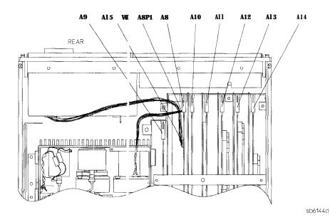
Figure 5-5. Power Supply Cable Locations
