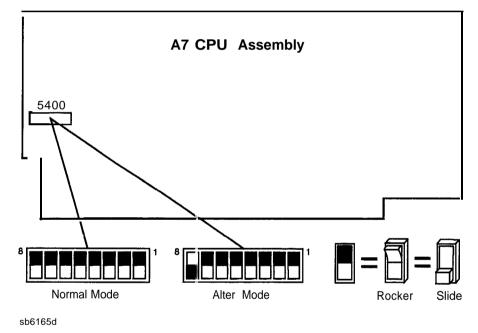
Figure 6-4. A7 Switch Positions (Firmware revisions 7.xx and above.)
