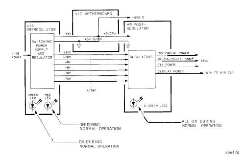
Figure 12-2. Power Supply Functional Group, Simplified Block Diagram
