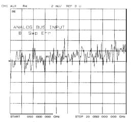
Figure 10-5. Node 8: Swp Err, Phase Error Voltage
