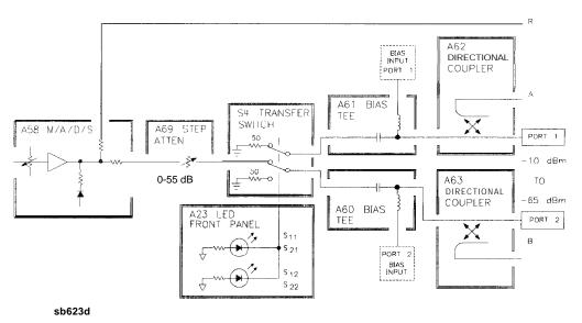
Figure 12-5. Signal Separation, Simplified Block Diagram
