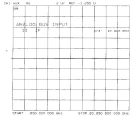
Figure 10-7. Location of Internal Counter Reading on Display
