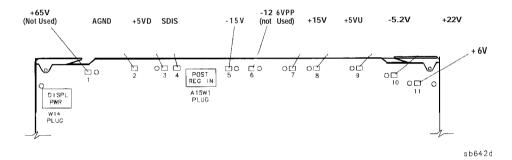
Figure 5-3. A8 Post Regulator Test Point Locations
