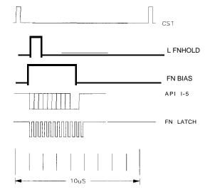
Figure 7-5. A14 TTL Signals at A14TP3
