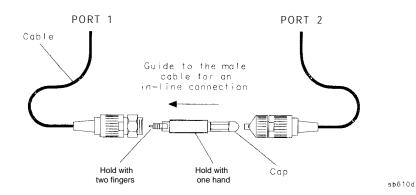
Figure 2-12. Aligning the Center Conductor
