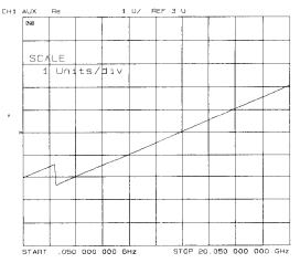
Figure 4-8. 0.25V/GHz Waveform at Abus Node 9
