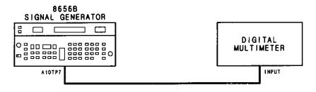
Figure 5-24. DC FM Offset Adjustment Setup
