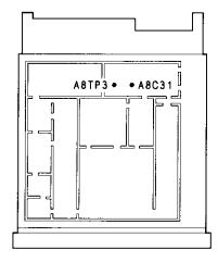
5. Tune the measuring receiver to the frequency of the Signal Generator and adjust A8C31 (PEAK ADJ) for a maximum RF Power reading.
