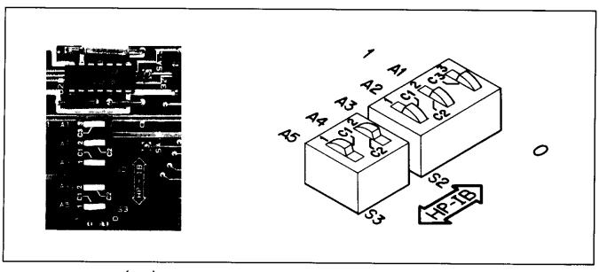
HP-IB Figure 2-3. HP-IB Address Switch Location and Settings
