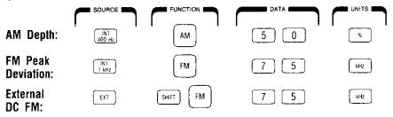
Internal, external, or mixed AM or FM functions can be selected. Modulation parameters are selected in the Source-Function-Data-Units format as shown in the examples above. One of the two internal modulation sources (400 Hz or 1 kHz) and/or a signal or dc level from an external modulation source coupled through the front-panel connector may be used to modulate the carrier.
