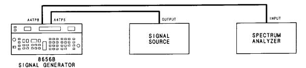
Figure 5-6. Notch Filters Adjustment Setup
