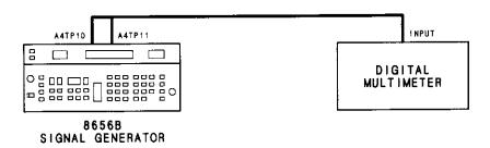
Figure 5-5. 715 MHz Sideband Adjustment Setup
