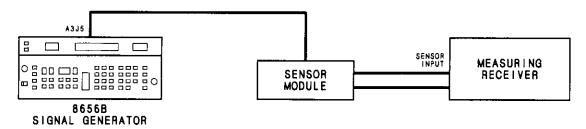
Figure 5-10. 50 MHz Reference Oscillator Level Adjustment Setup
