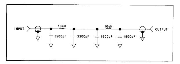
Figure 4-6. IMHz Low-Pass filter
