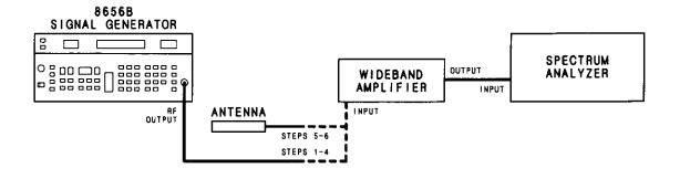
Figure 4-11. Output Leakage Test Setup
