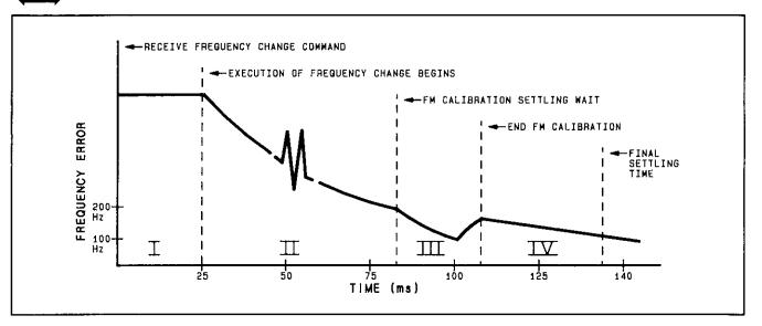
Figure 3-6. Frequency Switching Characteristics
