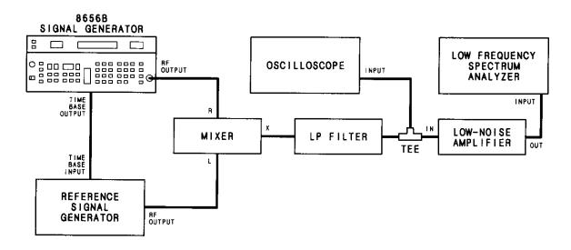
Figure 4-5. SSB Phase Noise Test Setup
