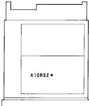
4. Adjust A10R52 (DC FM OFFSET ADJ) for a frequency counter reading of 65.000000 MHz ±10 Hz.
