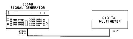
Figure 5-2. +2 Vdc Reference Adjustment Setup
