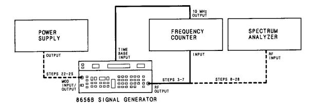
Figure 3-3. Test Setup for Basic Functional Checks
