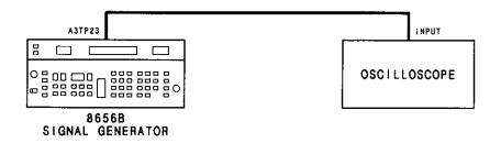
Figure 5-18. FM Calibration Pretune Adjustment Setup
