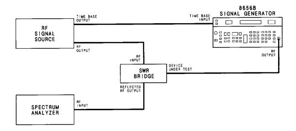
Figure 4-12. SWR Performance Test Setup (Out of Band)
