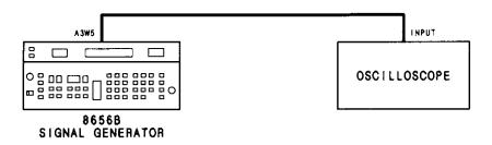
Figure 5-20. Pedestal Adjustment Setup
