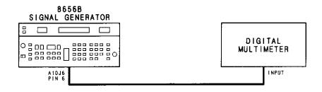
Figure 5-3. Audio Oscillator Level Adjustment Setup
