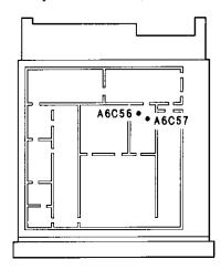
4. Tune the measuring receiver to the Signal Generator frequency by pressing the FREQ key. Press the RF POWER key and adjust A6C56 (ACC ADJ) for a 0 dBm ±0.5 dB reading on the measuring receiver.
