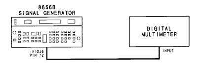
Figure 5-4. AM Offset Adjustment Setup
