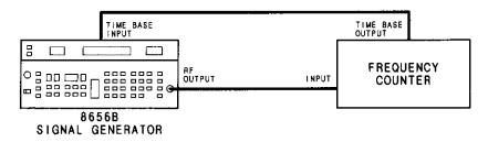
Figure 5-25. DC FM Frequency Offset Adjustment Setup
