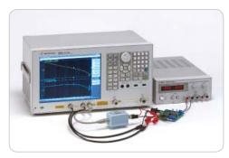
*DC-DC* converter loop-gain measurement with gain-phase test port
