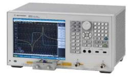
Gain-phase series-thru method using 16047E 4TP type fixture
