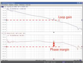
DC-DC loop-gain measurement
