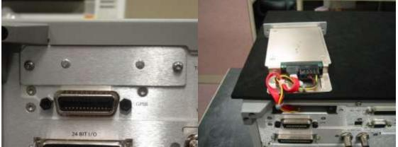
4. Disconnect both connectors from the HDD, and then remove the four screws holding the hard drive to the case.
