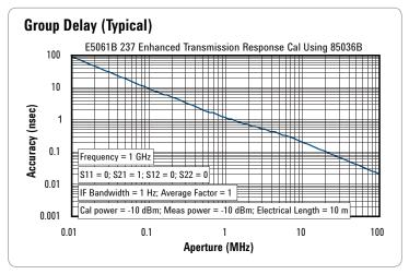
In general, the following formula can be used to determine the accuracy, in seconds, of specific group delay measurement:  $\pm$ phase accuracy (deg)/[360 x aperture (Hz)]
