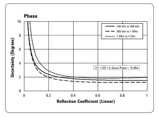
Table 9. . Corrected system performance with Type-N 75  $\Omega$  connectors, 85036B calibration kit, enhanced response calibration
