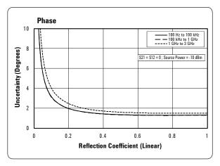
Table 3. Corrected system performance with Type-N 50  $\Omega$  connectors, 85032F calibration kit, enhanced response calibration
