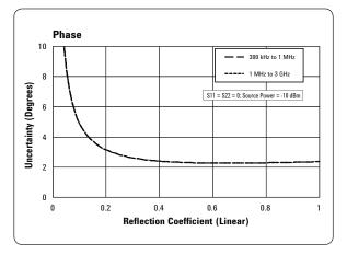
Table 8. Corrected system performance with Type-N 75  $\Omega$  connectors, 85036B calibration kit, full 2-port calibration
