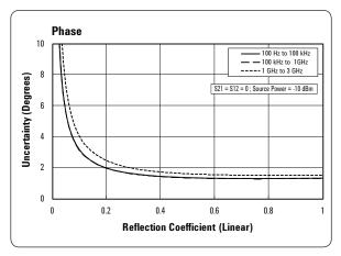
Table 4. Corrected system performance with Type-N 50  $\Omega$  connectors, 85092C ECal Module, full 2-port calibration
