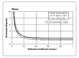
Table 7. Corrected system performance with Type-N 50  $\Omega$  connectors, 85092C ECal Module, full 2-port calibration
