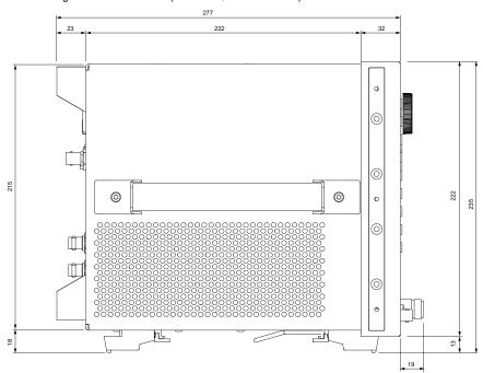
Figure 23. Dimensions (side view, in millimeters)
