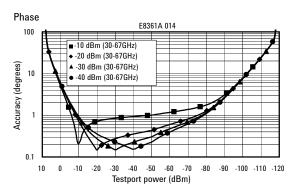
Dynamic accuracy is verified with the following measurements: compression over frequency, IF linearity at a single frequency of 1.195 GHz and and a reference level of -20 dBm for an input power range of 0 to -120 dBm.
