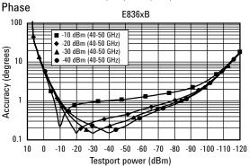
Dynamic accuracy is verified with the following measurements: compression over frequency, IF linearity at a single frequency of 1.195 GHz and a reference level of -20 dBm for an input power range of 0 to -120 dBm.
