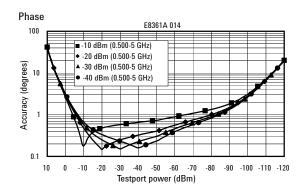
Dynamic accuracy is verified with the following measurements: compression over frequency, IF linearity at a single frequency of 1.195 GHz and and a reference level of -20 dBm for an input power range of 0 to -120 dBm.
