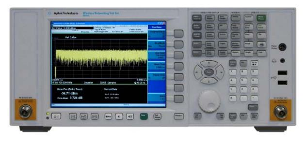
The Agilent N8300A wireless networking test set is a onebox radio frequency (RF) parametric test set based on an architecture that includes an integrated vector signal analyzer (VSA) and a vector signal generator (VSG). The Agilent N630XA measurement applications add onebutton measurements and modulation analysis capabilities to help with your design, evaluation, and manufacturing test of WiMAX<sup>™</sup> and WLAN (Wi-Fi) devices and modules.
