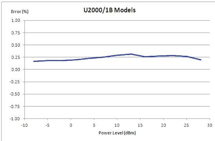
Typical power accuracy at 25 °C for U2000/1/2H sensors<sup>1, 2</sup>
