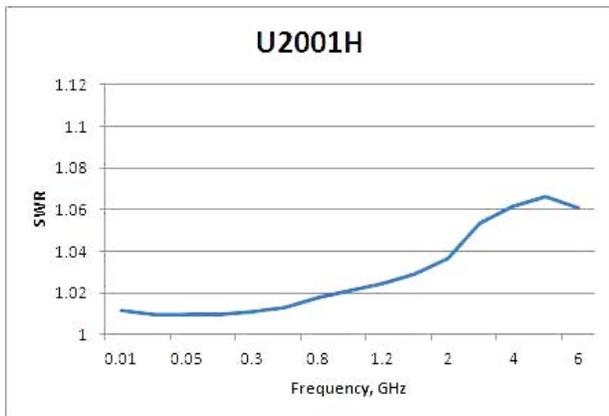
Typical SWR for U2001H sensor (25 °C ± 10 °C)
