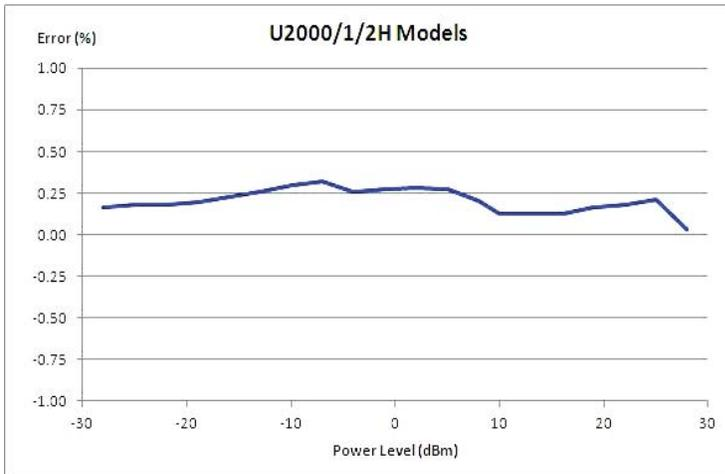
1. Measurement uncertainty  $\leq 1.9\%$ . At room temperature and excluding power level dependent terms (zero set, drift, and noise). Refer to Agilent Fundamentals of RF and Microwave Power Measurements (Part 3) Power Measurement Uncertainty per International Guide (Application Note 1449-3), 5988-9215EN for more information on measurement uncertainty.
