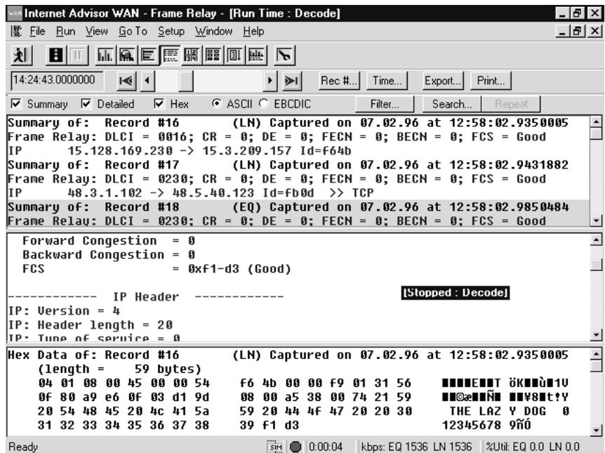
Figure 1. The HP Internet Advisor fully decodes frames and cells, and displays all fields.
