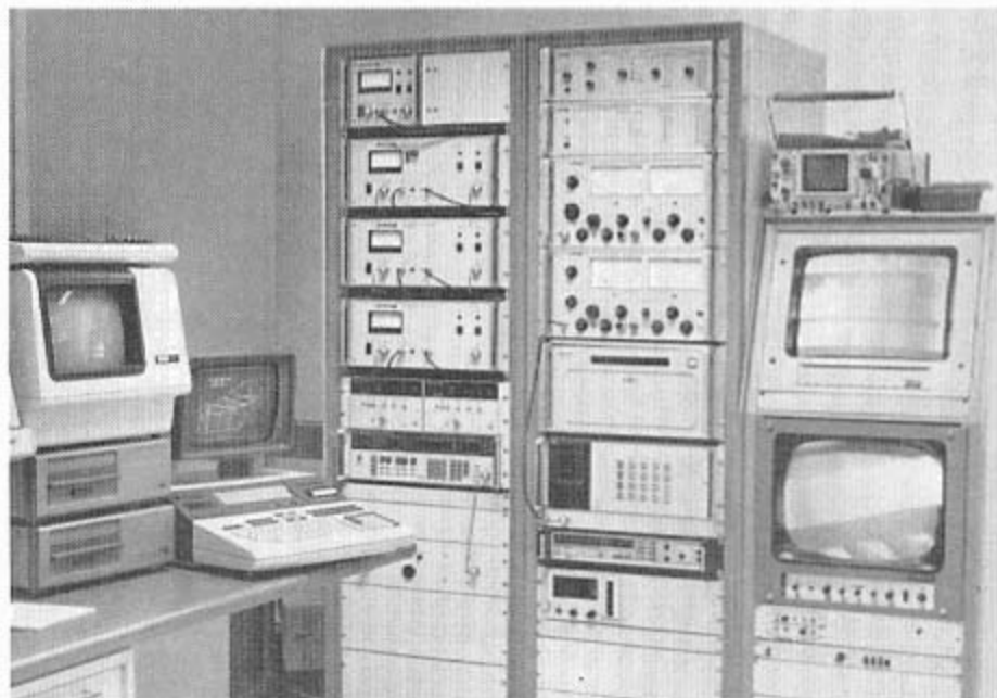
Eaton Broadband Amplifiers in use as a source for susceptibility testing systems.
