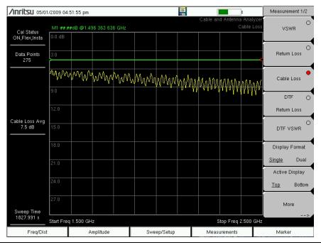
Figure 2-12. Cable Loss Measurement
