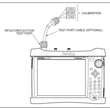
Figure 3-1. Calibration Setup OSL Cal
