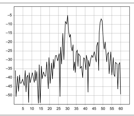
Figure A-1. Rectangular Windowing Example
