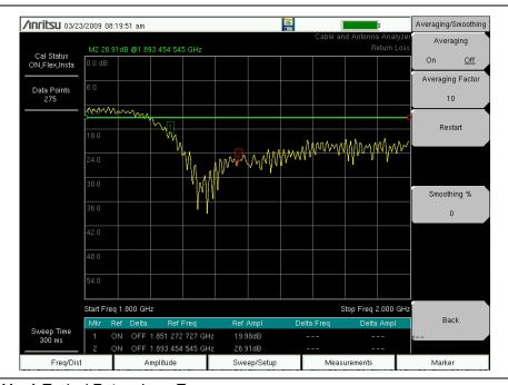
Figure 2-11. A Typical Return Loss Trace
