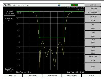
Figure 2-4. Segmented Limit Lines
