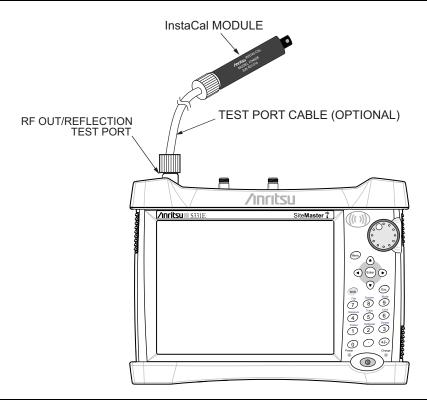
Figure 3-2. Calibration Setup InstaCal
