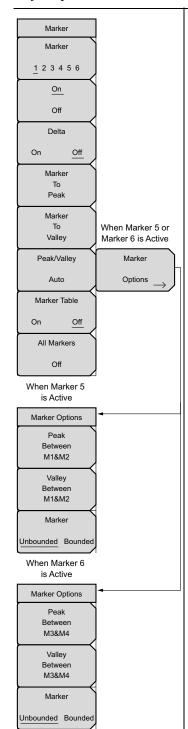
**Marker:** Press the marker key the select M1 to M6 on the touch screen to choose the active marker. The underlined marker number is the active marker.
