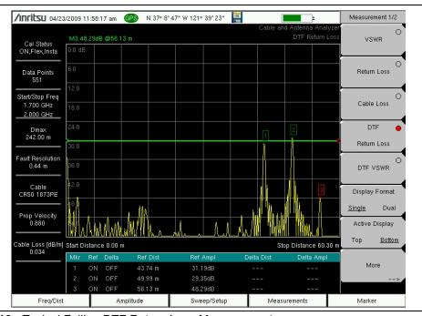
Figure 2-16. Typical Failing DTF Return Loss Measurement
