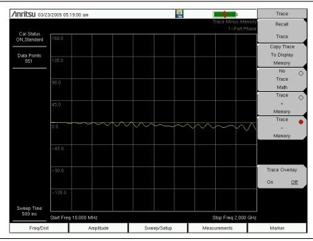
Figure 2-9. Trace-Memory Used to Compare the Phase of Two Cables
