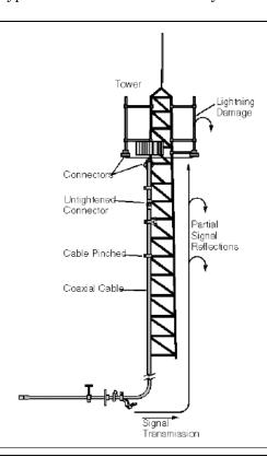
Figure 2-10. A Typical Transmission Feedline System
