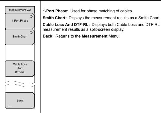
Figure 2-28. Measurement Menu (2 of 2)
