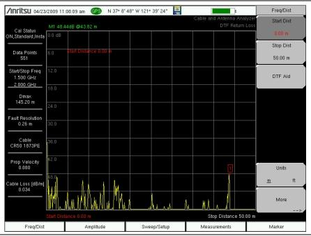
Figure 2-15. Typical Passing DTF Return Loss Measurement
