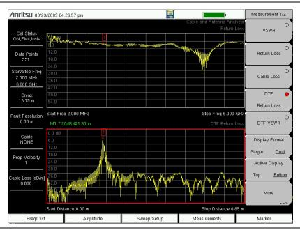
Figure 2-2. Dual Display with the Bottom Display Active
