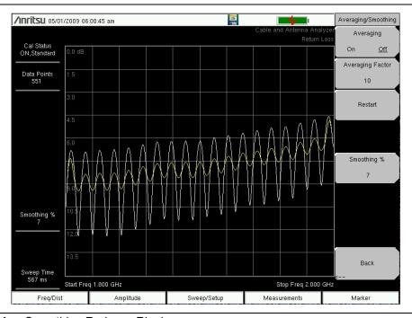
Figure 2-1. Smoothing Reduces Ripple
