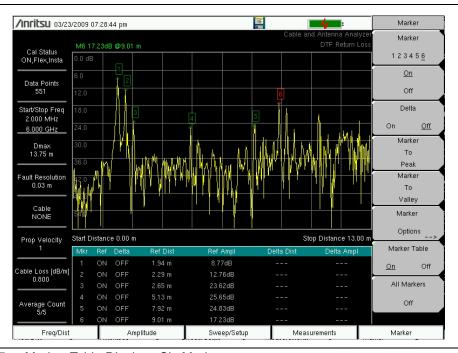
Figure 2-7. Marker Table Displays Six Markers
