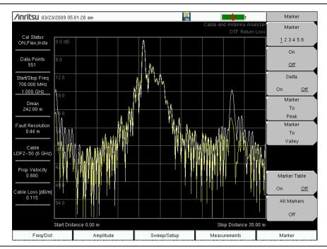
Figure 2-8. Trace Overlay of Two DTF Traces
