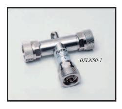
The OSL series open/short/load are used on the test port of the Site Master Series of handheld instruments to establish a reference for accurate measurement. When used with a Site Master, the open/short and load reflection over a swept frequency range can be automatically averaged to enhance measurement accuracy. OSL series Open/short/load comes in both N(Male) and N (Female) connector configuration and consist open on one end, short on other and Load on the tee section.
