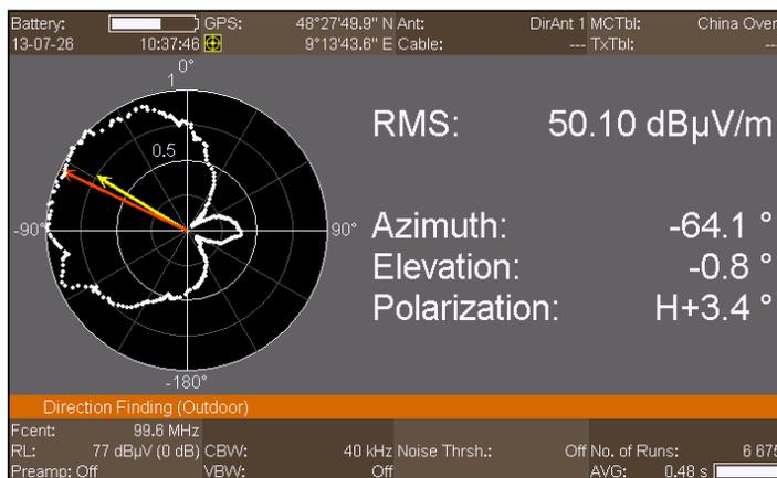
**A Horizontal Scan, i.e. taking bearings all round, at a frequency of 99.6 MHz and a bandwidth of 40 kHz. The result is shown as a polar diagram. The red arrow indicates the maximum and hence the suspected direction of the interference source.**
