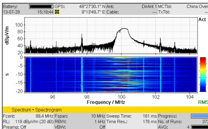
**A single spectrum (above) taken from the spectrogram (below).** The time characteristic can be followed by retrieving the individual spectrums one after the other.
