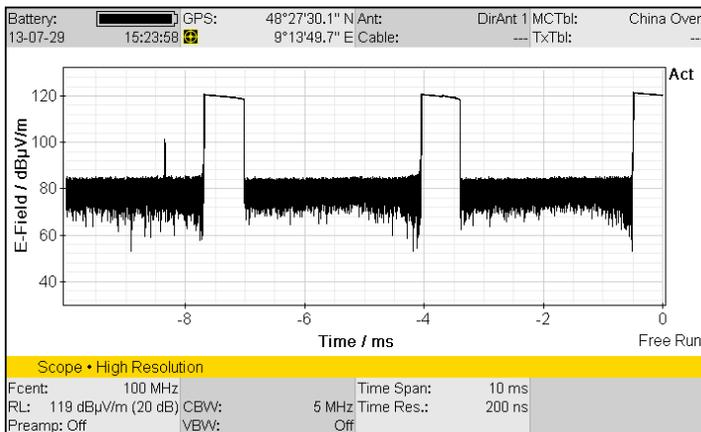
*Direct examination of the defective device. Scope mode shows the time characteristic of the interference signal level exactly.*
