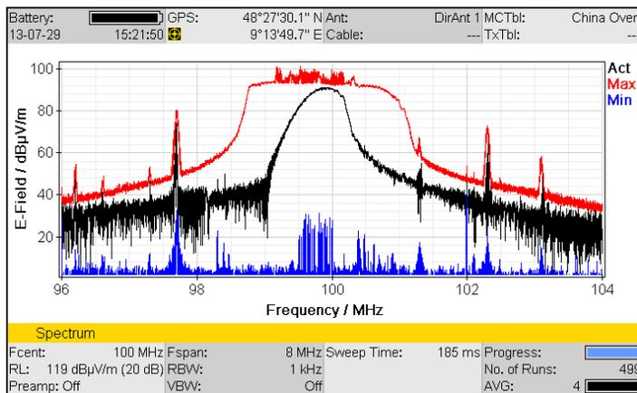
**Spectrum mode.** The type of interference becomes clear when you display the actual, maximum and minimum levels.
