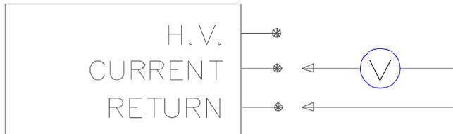
The instrument will automatically provide 10 volts AC across the voltmeter upon pressing the 0 key on the numeric keypad. The ■ G-TEST led will come on. The displays will then be similar as below:
