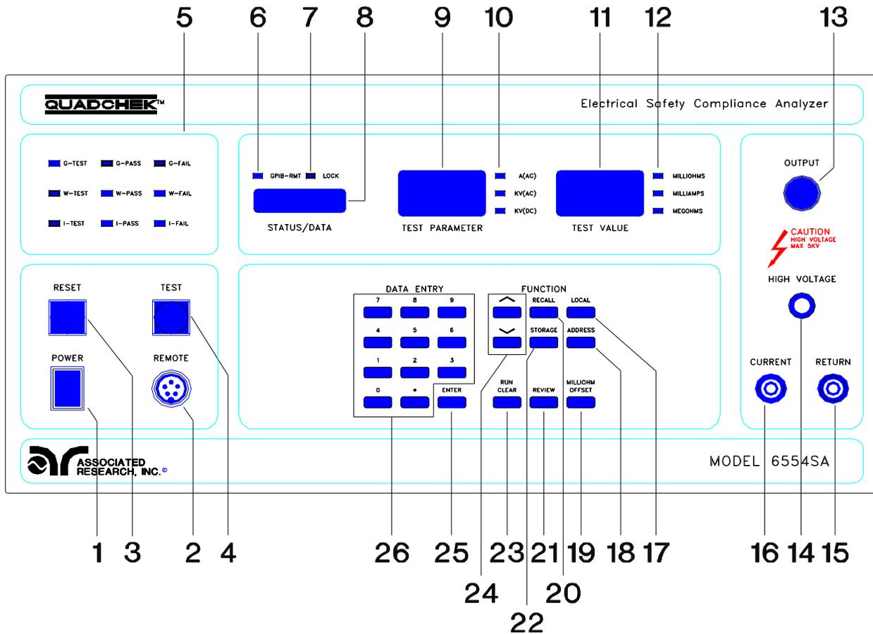
9. **TEST PARAMETER LED WINDOW:** This is a numeric display of test parameters or results for ac current, ac voltage or dc voltage.
