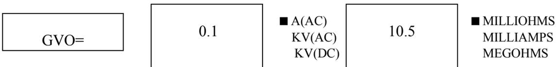
Please key in the reading on the Voltmeter into the instrument via the numeric keypad in units of 10mV. For example: If the reading on the Voltmeter is 10.12 volts you would press 1 0 1 2 ↵ “ENTER”. The AC Voltage is then calibrated. You will be returned to the main calibration display.
