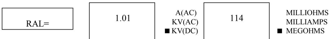
Please enter the reading on the microammeter into the instrument in units of  $0.01 \mu\text{A}$ . For example: If the reading is  $9.92 \mu\text{A}$  then enter 9 9 2 ENTER ↵. The high range of the insulation measuring circuit is calibrated and you are returned to the main calibration screen.
