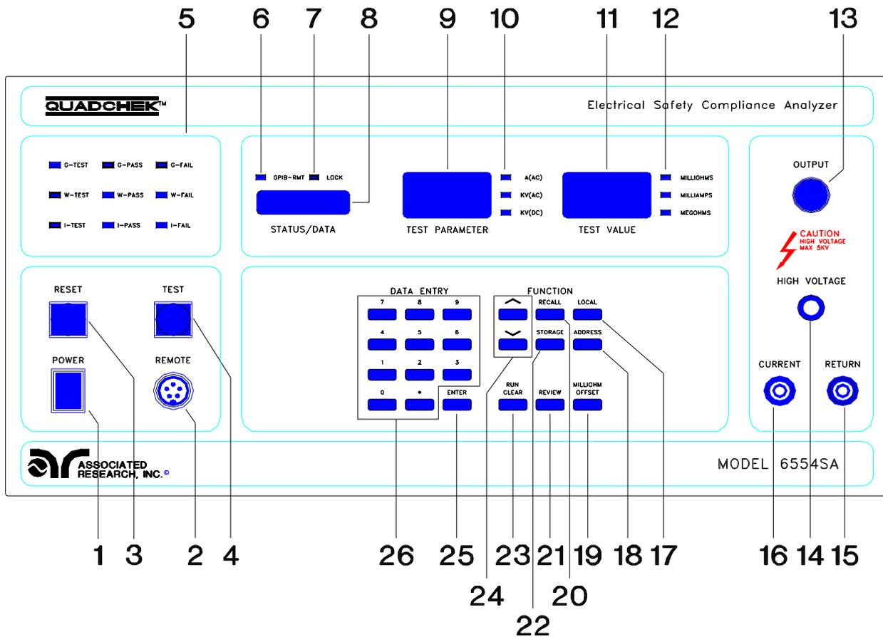
4. **TEST SWITCH:** This is a momentary contact switch. Press the blue switch to turn on the high voltage output.
