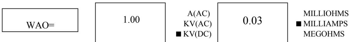
Current will then flow through the ammeter. Please enter the reading of the ammeter into the instrument in units of 0.01 mA. For example: If the reading of the ammeter is 8.27 mA, then you would enter 8 2 7 ENTER ↵. The leakage current is then calibrated and you will be returned to the main calibration screen.
