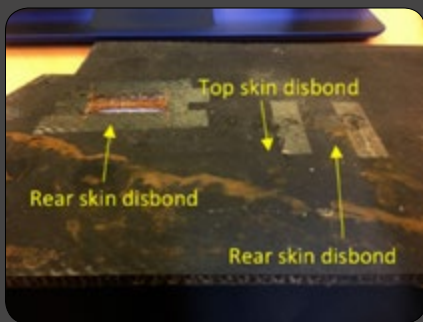
Figure 3: Thin CFRP honeycomb sample with rear surface disbands.
