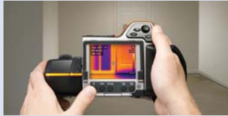
Infrared cameras quickly locate moisture related problems
