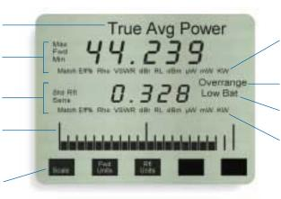
Measurement Units for Major Digital Display (Select with Speed Key)
