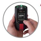
A: Use the up and down arrows to navigate to bump test or calibrate from gas options in the main menu From there, follow the instructions on G7 screen
