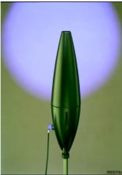
Fig. 6 OmniSource Sound Source Type 4295
