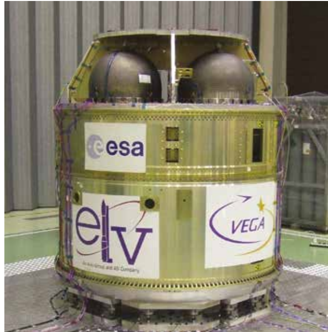
ESA's VEGA launcher upper-stage being tested on the LDS QUAD Shaker System, at the European Space Research and Technology Centre (ESTEC), in The Netherlands. (Image courtesy of ESA, 2009)
