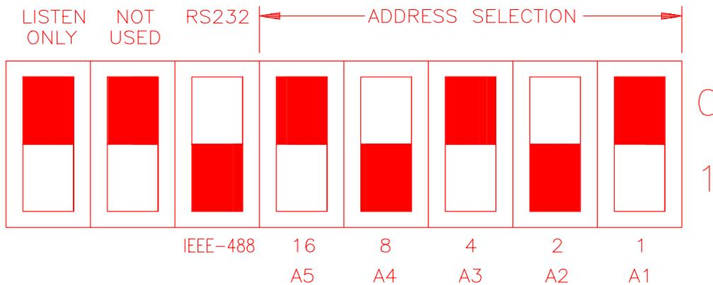
Figure 8-2: GPIB Address Selection Switch
