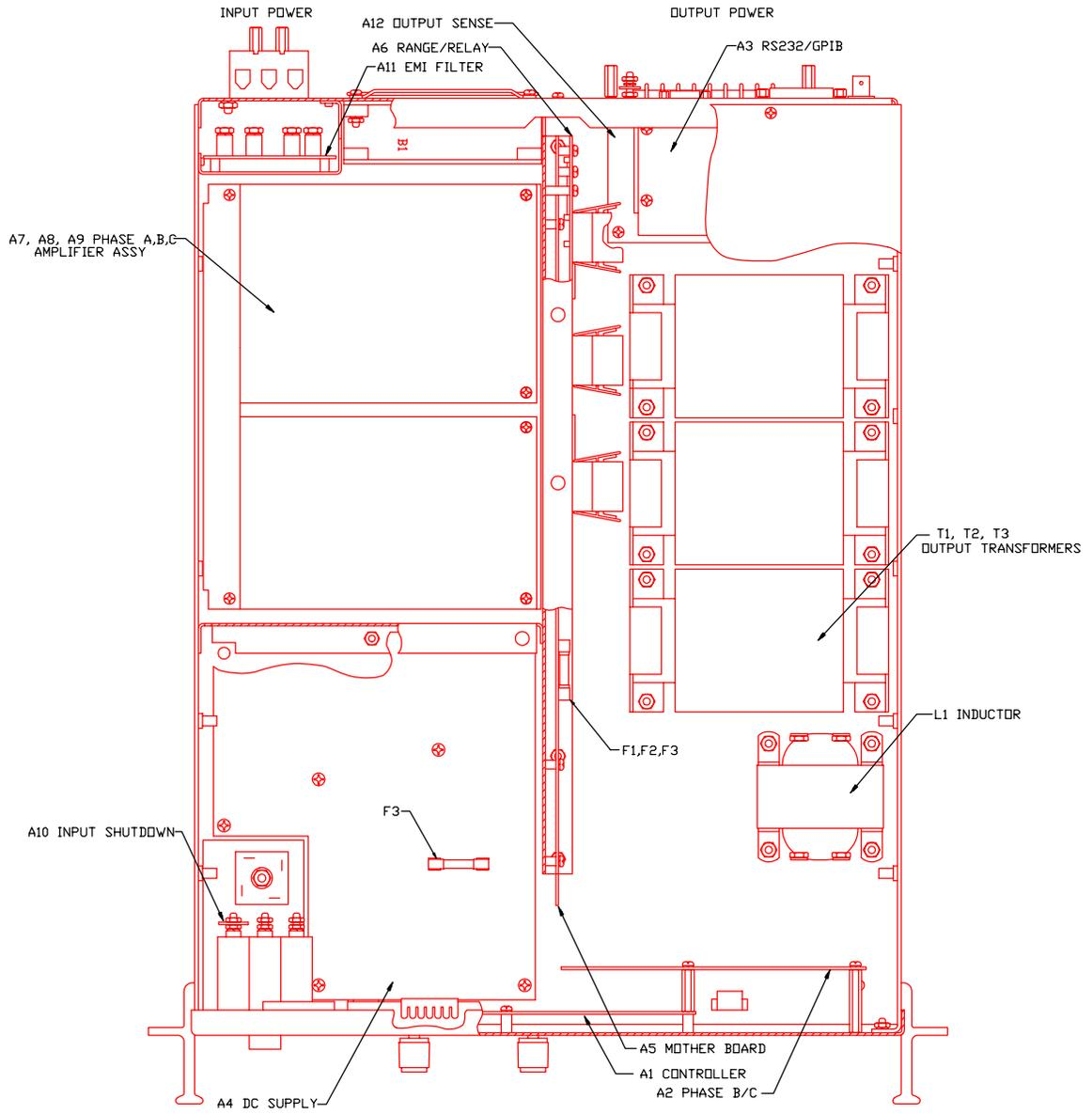
Figure 7-1: Assembly Location
