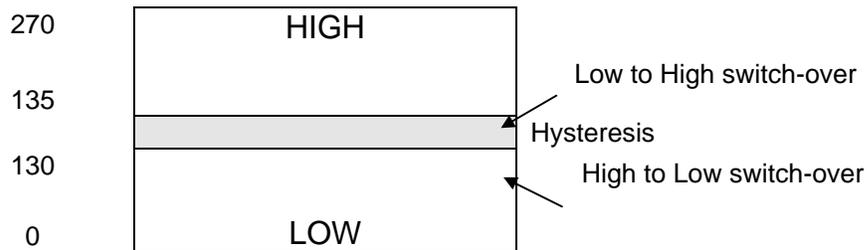
Figure 4-2: Voltage Auto Range Switch Over Points
