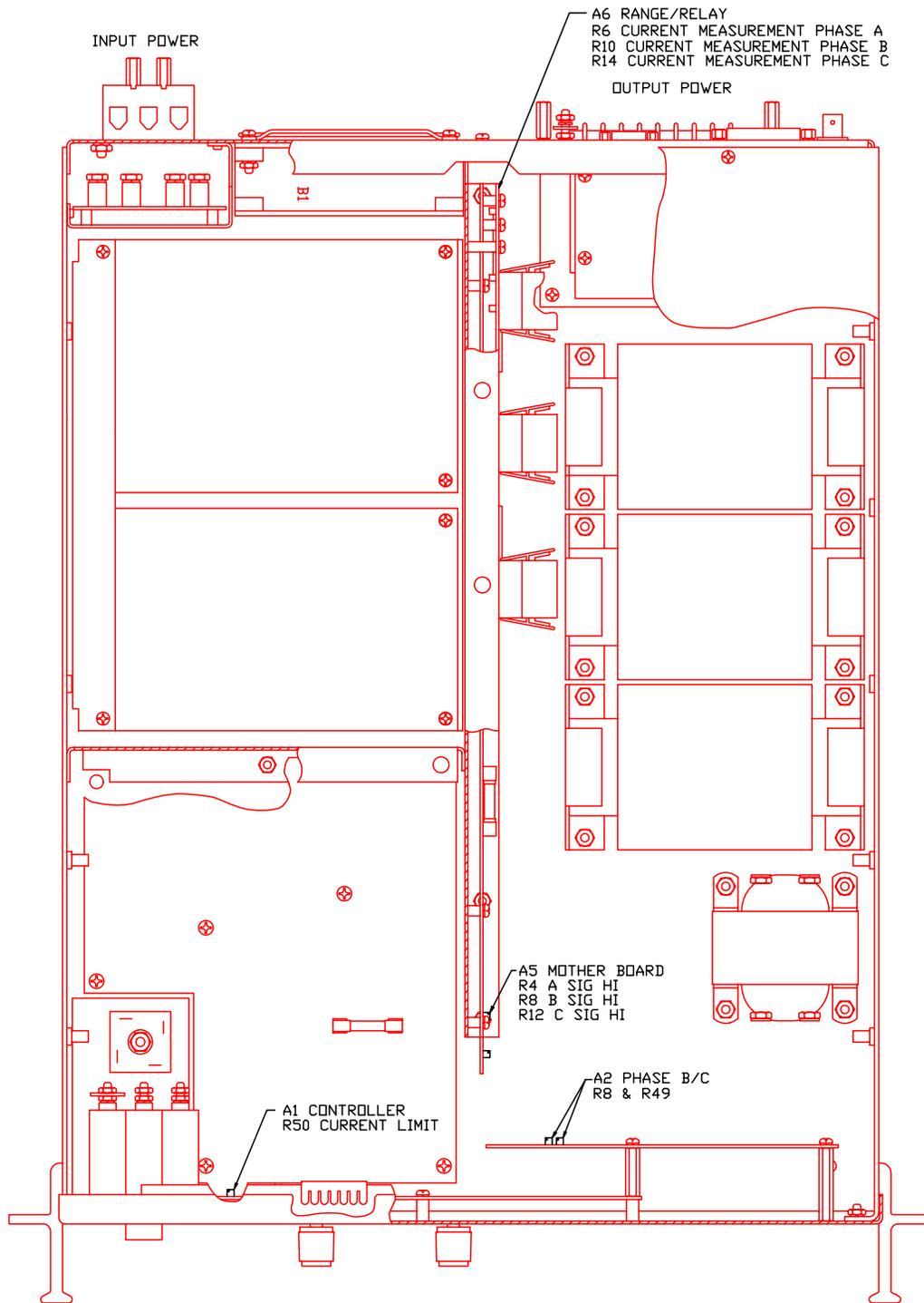
Figure 6-3: Internal Adjustments
