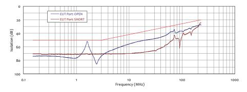
Data shown on above graphs is representative of a typical CDN M325E Coupling/Decoupling Network.
