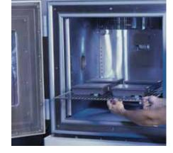
• The workspace interior is heliarc-welded with type 304 brushed stainless liner that is easy to clean
