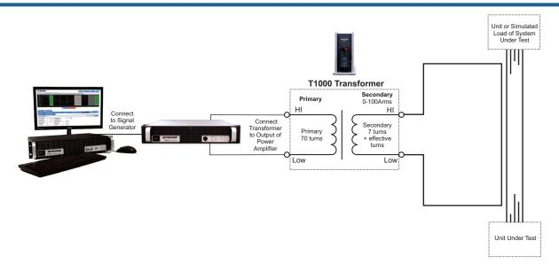
Figure 2 – Sample Application: DO 160 Section 19 Test Load Wiring
