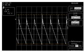
Figure 3 – Example of output from the CR 600 when adjusted for a repetition period of 0.2 to 10 microseconds
