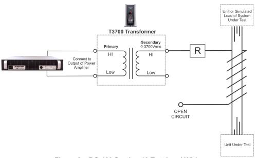
Figure 2 - DO 160 Section 19 Test Load Wiring
