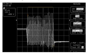
Figure 2 – Example of output from the CR 600 when adjusted for a pulse sequence with an amplitude greater than or equal to 600 Vpp, and a total duration of 50 to 1000 microseconds
