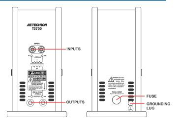
Figure 4 - T3700 Controls and Connectors
