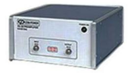
The Com-Power PA-010 is a general purpose, broadband, high gain, bench top preamplifier. The PA-010 reduces floor noise and increases system sensitivity to low level signals during Electromagnetic Interference (EMC) testing. It also provides input isolation to your expensive test equipment. The PA-010 operates from 100 Hz to 30 MHz.
