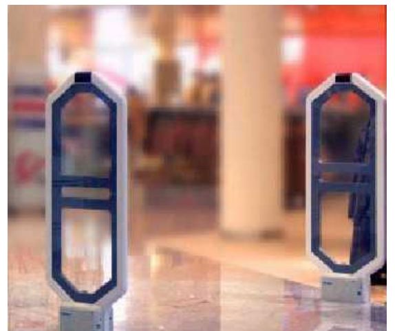
Magneto acoustic gate used for product surveillance
