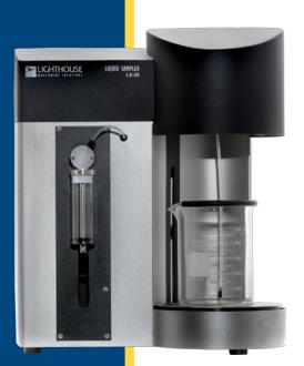
THE LS-20 Liquid Sampler has an integrated syringe sampler and optical particle counting system. It's easy-to-use Windows<sup>tm</sup> based software interface is designed to meet the international regulatory EP and JP, as well as USP 788 requirements.
