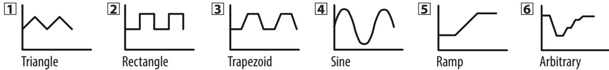
Additionally to the standard functions, which are all based upon a so-called arbitrary generator, this base generator is accessible for the creation and execution of complex sets of functions, separated into up to 99 sequences. Those can be used for testing purposes in development and production. The sequences can be loaded from and saved to a standard USB stick via the USB port on the front panel, making it easy to change between different test sequences.
