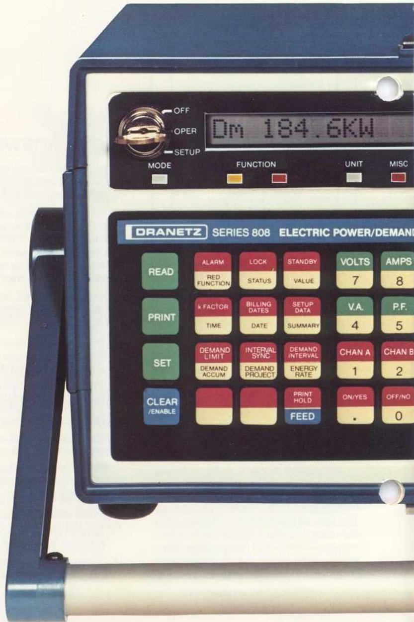
The Series 808 will accommodate the demand interval schedules used by any power company. The operator can easily set fixed time intervals from 1 to 120 minutes in one minute increments or sliding intervals from 5 to 60 minutes in five minute steps with overlapping five minute increments. Either internal or external synchronization can be selected.
