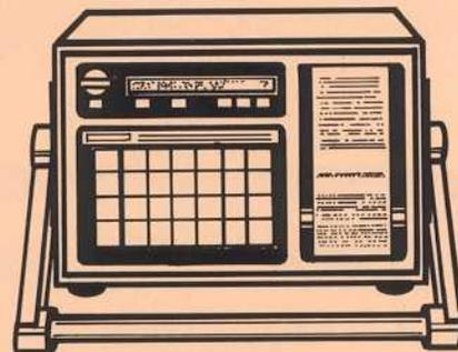
One Series 808 can control all setups and data outputs from any other Dranetz analyzer with communications capability.
