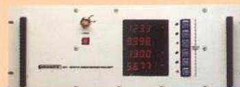
*The Model 810 Remote Power/Demand Analyzer* incorporates the capabilities of the Model 808 with its communications interface, mounts in a 19-inch rack and is designed to operate in severe RFI and EMI environments. The front panel includes a security keyswitch and its LED indicator.
