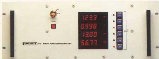
**Models 809 and 810**—Designed for permanent, rack mounted installation, the 809 Remote Power/Demand Analyzer provides remote monitoring of power usage in industrial, commercial, and electric utility applications. A built-in 32K character buffer memory, RS-232C port and Bell 103 compatible modem
