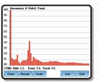
can cause small, almost imperceptible variations in performance that aggregate to effect significant long-term damage. Current harmonics generated by a source can pollute the entire power system without being affected itself. The PowerXplorer captures detailed harmonics, interharmonics and subharmonics to effectively troubleshoot the complex problems caused by these events.
