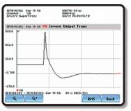
switching, lightning, transformer energization, and load shifting, are immediately characterized as impulsive or oscillatory and detailed for further analysis. Capable of capturing the complete power quality spectrum, the PowerXplorer provides scope-like display of the entire transient.
