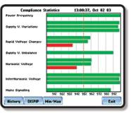
quality-of-supply standards and benchmark power quality. In an instant, the PowerXplorer provides a snapshot of over 13 key parameters, including unbalance, voltage variations and harmonics.
