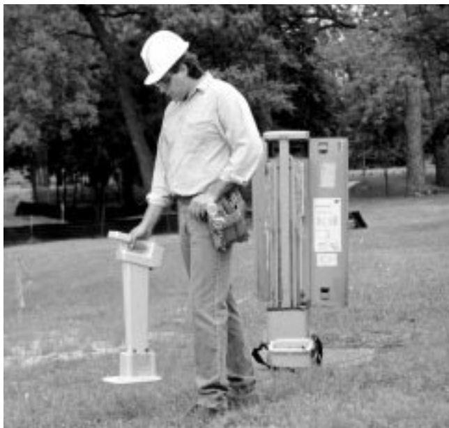
The Dynatel 2250 Cable Locator can be used with the Dynatel 2205/2206 EMS Marker Locating Accessory.
