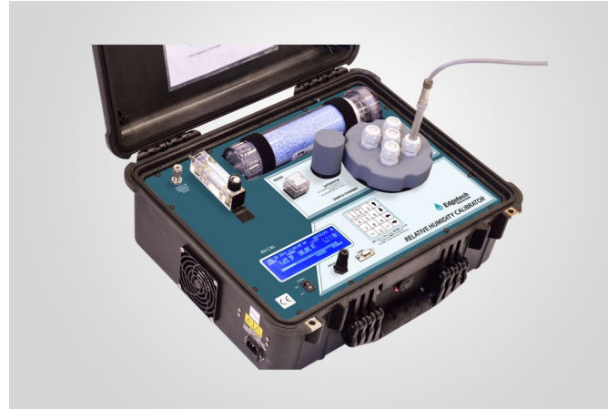
RH CAL with Probe Inserted for Calibration Through Port Into Sample Chamber
