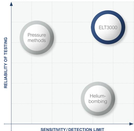
second not finding liquid leaks reliably. The answer to a reliable and at the same time very sensitive battery leak test is the ELT3000.
