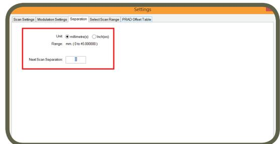
Simply enter the distance between the antenna and the surface of the scanner in millimeters or inches. The maximum separation value that you can enter for RFX is 45 mm and for RFX2 is 115 mm. The displayed limit will change automatically based on the connected hardware i.e. RFX or RFX2. The far-field calculation will be automatically adjusted to account for the increased distance.
