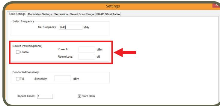
If you know the Conducted Sensitivity value of the DUT, RFxpert will estimate the TIS of the DUT without going through a time consuming test plan. You must first enable and complete the Source Power data fields.
