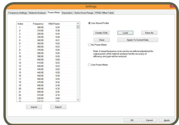
To create a profile automatically, simply enter the start, stop frequency and number of points. The output power must be within the limits of the network analyzer but typically should be the maximum allowed value. When you click the ‘Create Profile’ button you see the list being populated. If these values seem reasonable, click the OK button. You can use the profile immediately or save it by clicking on the Save As button.
