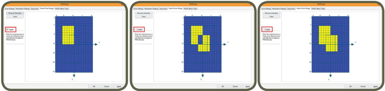
An example of using the measurement mask is shown here. You can see the mask settings as well as the impact it has on the near-field results. The masked area will never show up in the far-field pattern.
