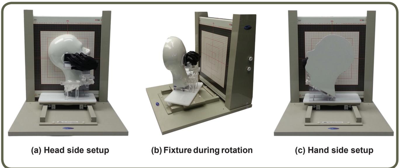
1. Place the head side next to the RFX2 scanner as shown in Figure (a). Be sure the head is right next to the scanner lid surface.
