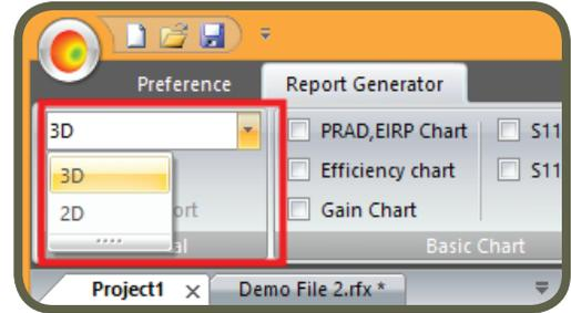
Each results window available in the RFExpert software is also available for the report generator. There are a total of 37 different results available. Some scan types will not have all 37 available if they are missing some of the required data for a scan type. Those will be grayed out in the report generator tab.
