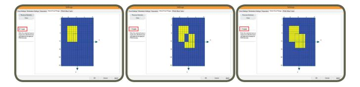
An example of using the measurement mask is shown here. You can see the mask settings as well as the impact is has on the near-field results. The masked area will never show up in the far-field pattern.
