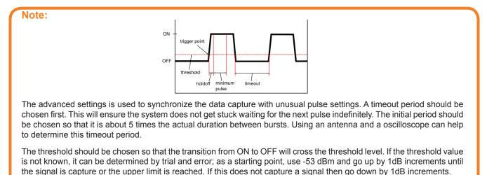
Once the hardware detects that the transmitted power has crossed the threshold level the system will wait for a holdoff period before beginning data capture. This holdoff period can typically be left at the default value unless the burst has a very slow rising envelope. After data capture has begun a minimum pulse duration of 500us is needed to ensure accurate measurement. Finally a timeout period can be specified.
