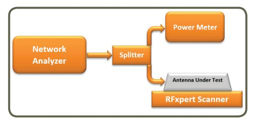
Power Meter Sensor and Power Splitter Setup
