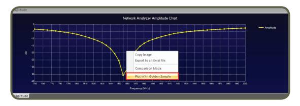
• Two plots of the S<sub>11</sub> scans will be superimposed with the red plot being the golden sample
