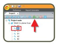
Repeat the movement in the y direction while running a scan every 40 cm at the appropriate node until all rows and columns are scanned. When all subscans are completed the parent node (Multi Co-Planar Scan) should automatically update. To view the results, first click on the parent node and then select the view: near-field or far-field.
