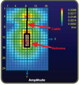
Fig. 8. Near-field emissions of the cable
