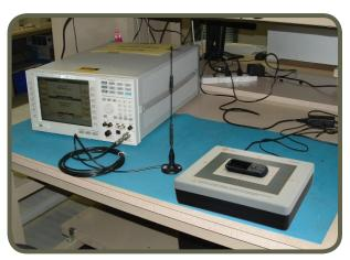
Enter all of the necessary parameters into the BSE to ensure a call can be established with the cell phone. Now a signal should be present for the base station to register the mobile. If the mobile cannot detect the BSE then base station power may have to be increased. Also consider the potentially high over the air path loss which could be 20-30 dB. Once the mobile has been registered, a call can be made to the mobile.
