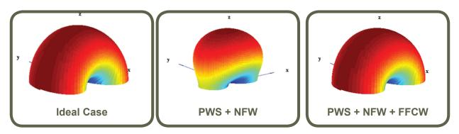
This The Radiation Pattern Correction is optimized for antenna elements in the center of the scanner. If the elements cannot be placed in the center of the scanner it may be better to process the data without the Near-Field Window. Significant near-fields within 5 cm of the center for the RFX2 and within 2 cm of the center for the RFX would be considered in the center.
