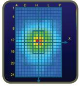
Client SW calculates far-field data based on near-field data in the background. If a project file is saved without checking Store with Dataset, client SW will not store the calculated far-field data and will calculate the far-field every time this file is opened.
