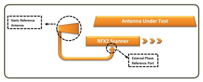
Once the phase port is set to external and the reference phase has been provided to the external phase port using the passive or active device method, you can go to scan settings.
