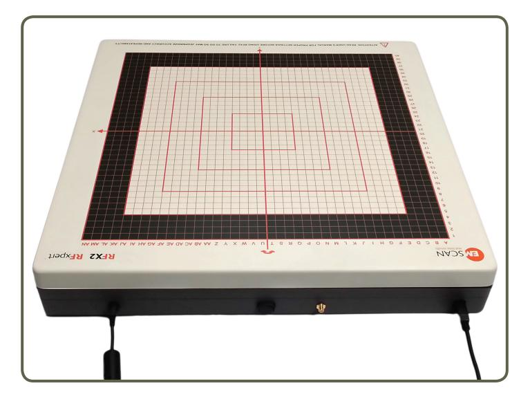
RFxpert Setup Showing Power and USB Cables (RFX2 model shown in the picture)
