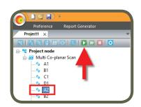
Repeat these steps until the first column is done. Return the RFX2 to the beginning position and then move it exactly 40 cm in the x direction to position B1. Run a scan for the first subnode of the second column in position B1.
