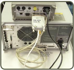
Network Analyzer and Power Meter Setup Showing Power and USB Cables
