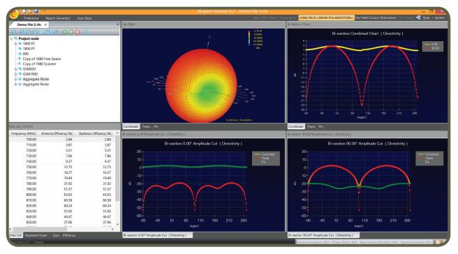
What is displayed is a full slice through the sphere that reflects a merging of two hemispheres (one for each side of the DUT). This merging will also apply to Bisection Polar View – Theta; and Bisection Polar View – Phi. TRP is also calculated.
