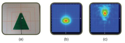
Fig. 5. (a) Log-periodic antenna on scanner (b) 1 GHz ~ 110 mm from end (c) 5 GHz ~ 0 mm from end
