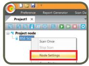
application until you see Base Station Emulator highlighted. To set scan settings for this scan type; first right click on the scan node and then left click on Node Settings to select between CDMA, GSM, WCDA and LTE nodes. Once you click on OK, the relevant Settings menu comes up.
