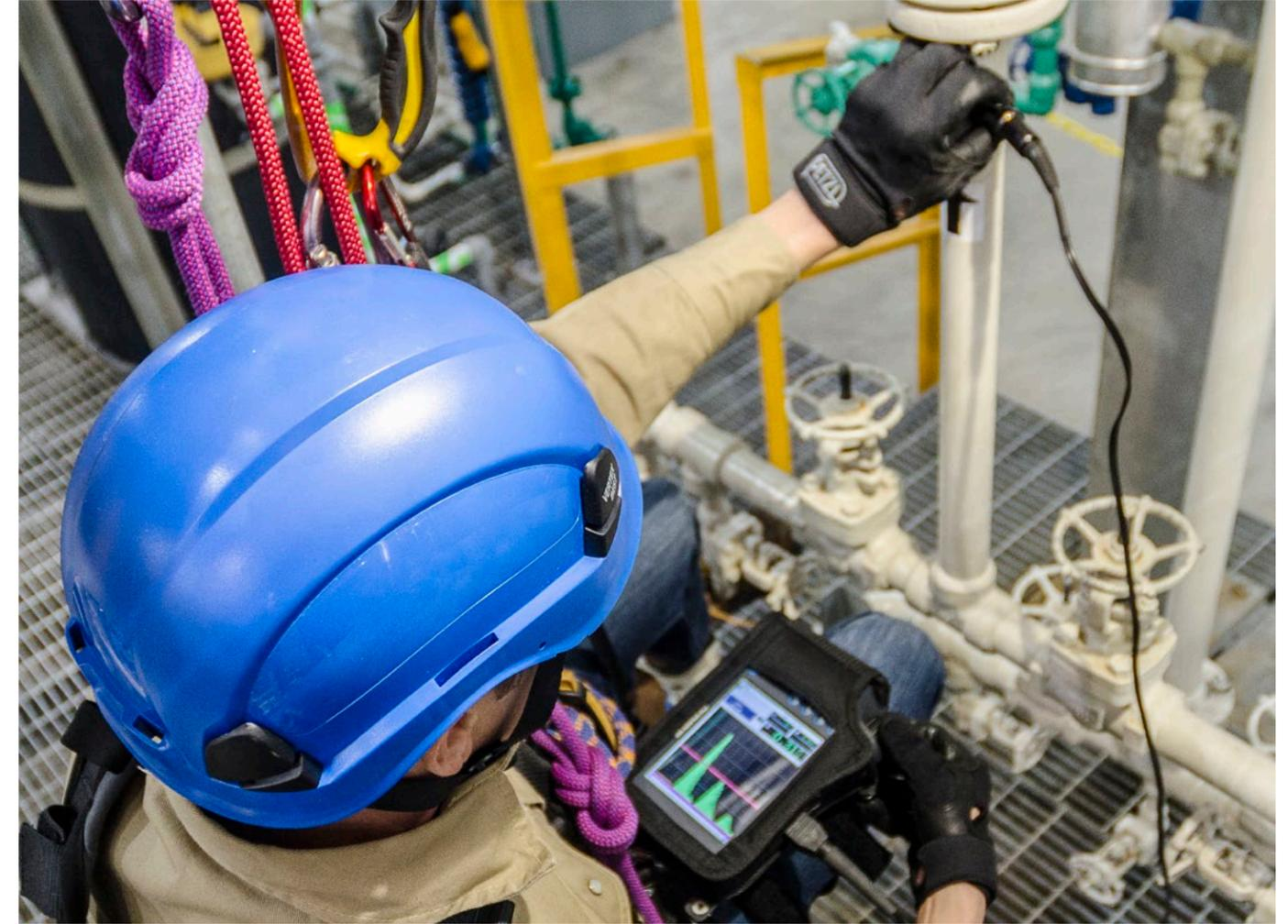
The workflow of the EPOCH® 6LT flaw detector is simple and straightforward. The primary screen is a large, optimized A-scan display that contains links to commonly used features and functions. Combined with an improved scanning workflow, users can complete their inspections with minimal button presses and adjustments. When you do need to navigate the menu, prominent icons make it easy to find the feature you're looking for.
