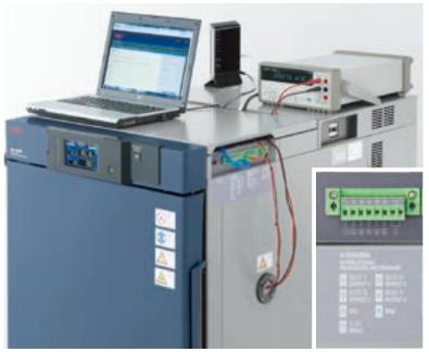
Instrumentation interlock terminals
