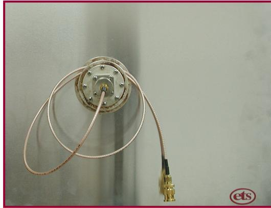
Figure 2.0-2: Compact Ground Plane Assembly
