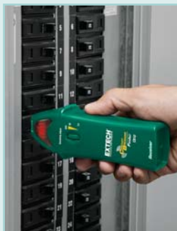
Adjustable sensitivity for pinpointing the correct breaker
