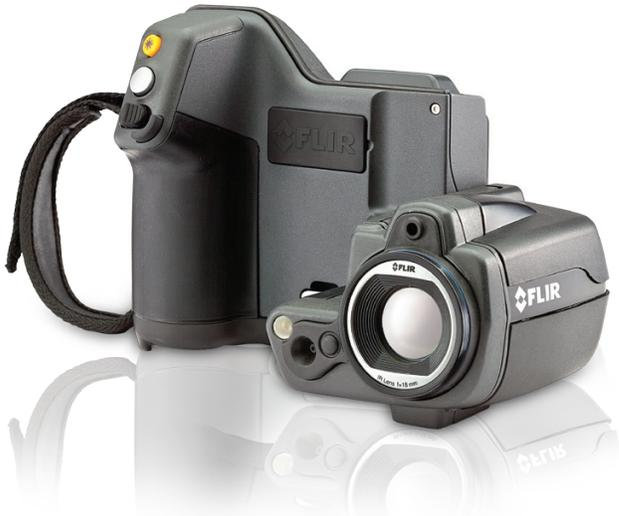
The FLIR T430sc is a thermal imaging camera with a rotating optical block and touch screen interface. This handheld camera is perfect for bench-top testing in the lab or dynamic testing in the field. The tiltable IR unit gives you great flexibility and allows you to conduct your experiments fast and in a comfortable position.
