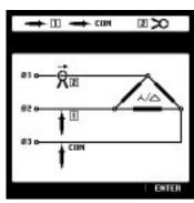
• **New!** On screen graphics show you how to set up 3-phase power measurements
