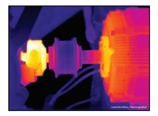
Identify a potential problem using a Fluke infrared camera.
