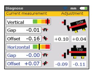
Corrective action using the Fluke 830 Laser Shaft Alignment tool.
