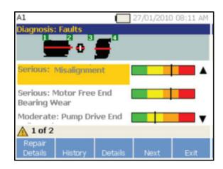
Diagnosis and repair recommendation using the Fluke vibration tool.
