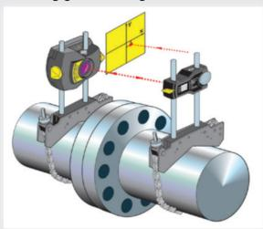
When machines are well outside of accepted tolerances, it can be difficult to get accurate alignment readings. For these gross misalignment problems, the Fluke 830 uses a unique "Extend" mode that enables better measurement accuracy by automatically increas-ing the effective sensor measurement area. Increasing the sensor measurement area virtually allows the Fluke 830 to address gross misalignment quickly without the need to perform an initial rough alignment.
