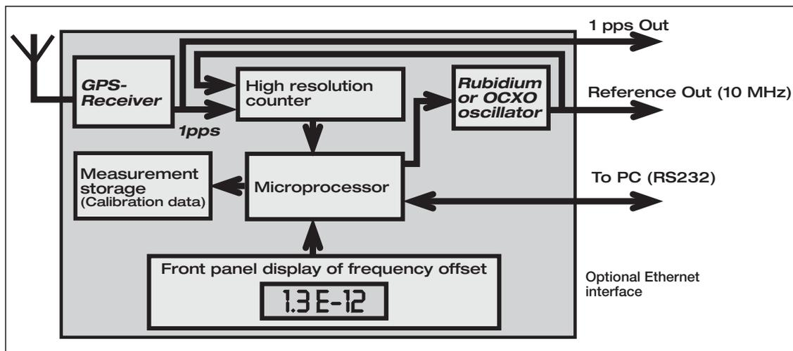
**Figure 2.** The Fluke Calibration 910 and 910R have built-in comparison between the GPS receiver and the internal oscillator. The frequency offset is displayed and stored and a traceability record can be produced at any time.
